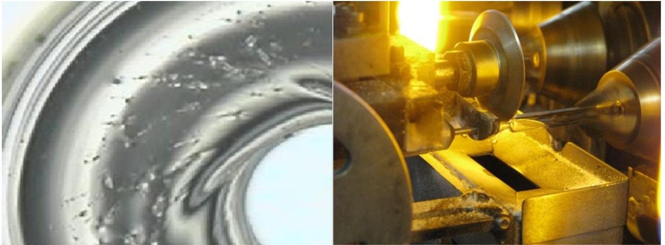
When these tiny air bubbles and rough surfaces come in contact with a surface contaminant, such as the lubricated on forming rolls and lure cone forming station, the contaminant is then transferred to the syringe tip. The contaminant, oil lubricant, is also inherent to the syringe manufacturing process. Oil lubricant must be used on forming rollers to avoid glass sticking to rollers.
