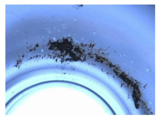
Though this flaw was initially characterized as "Minor" because of the lack of patient safety impact, the pharmaceutical manufacturer implemented a 100% pre-use visual inspection of all syringe barrels received. This inspection was to remain in place until such time as corrective actions could be proven effective at reducing the occurrence of the black spot flaw to acceptable levels.
