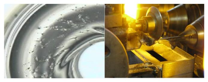
When these tiny air bubbles and rough surfaces come in contact with a surface contaminant, such as the lubricated on forming rolls and lure cone forming station, the contaminant is then transferred to the syringe tip. The contaminant, oil lubricant, is also inherent to the syringe manufacturing process. Oil lubricant must be used on forming rollers to avoid glass sticking to rollers.
